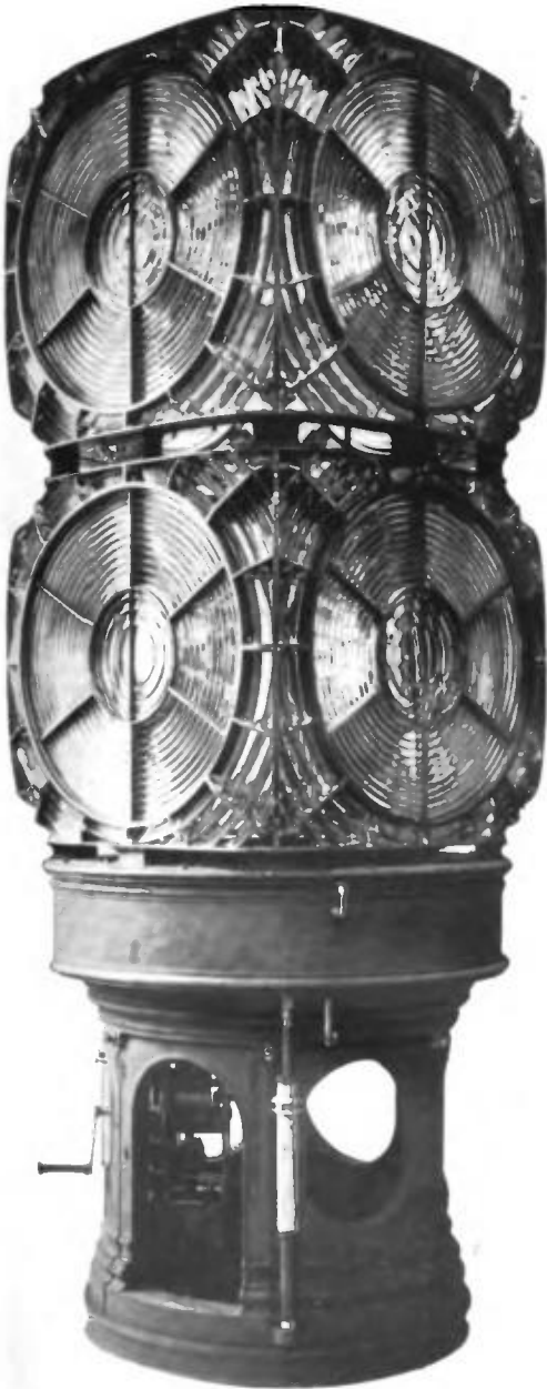
Fig. 54.—Fastnet Lighthouse—First Order Single-Flashing Biform Apparatus.
