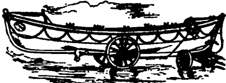
FIG. 1.—The 33-ft., Double-beaked, Ten-oared, Self-righting and Self-emptying Life-boat (1881) of the Institution on its Transporting Carriage, ready for launching.
