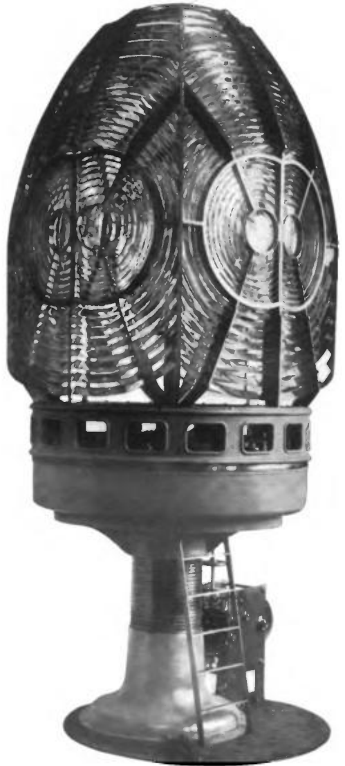
Fig. 55.—Pachena Point Lighthouse, B.C.—First Order Double-Flashing Apparatus.
